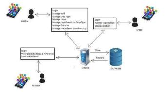
Fig -4.1: System Architecture of Crop Prediction System
